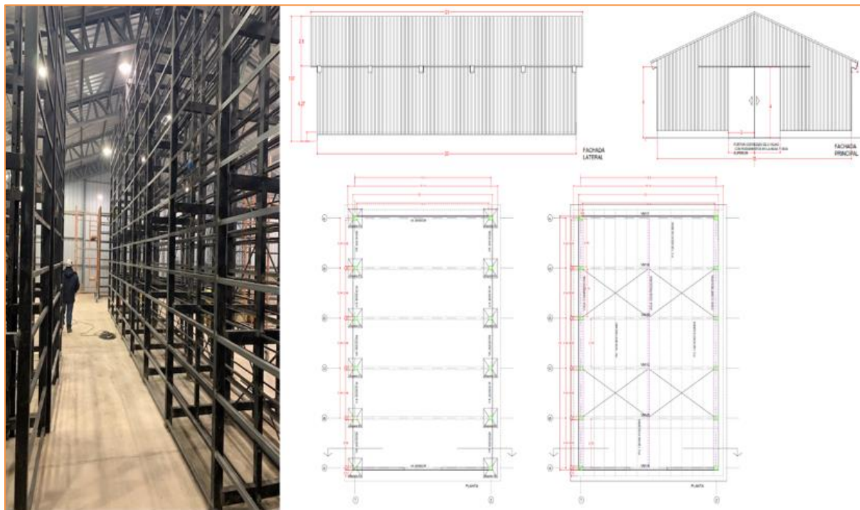
Figure 18-43: Core Storage Building and Racks for Approx. 30,000 m of Cores.
