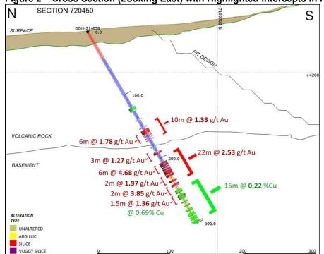
Figure 2 – Cross Section (Looking East) with Highlighted intercepts in Hole DDH 21-058
